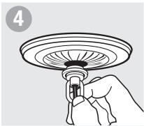
Cover with canopy and secure with screw collar loop.
