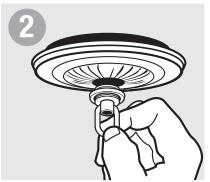
Check fit, cover outlet box with canopy and secure with screw collar loop. If needed, adjust nipple so canopy rests against ceiling after installation. Remove.
