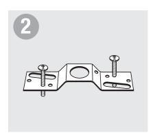
On raised side of crossbar, thread mounting screws down through each hole that lines up with canopy.
