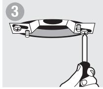
With raised side of crossbar towards ceiling, mount crossbar by inserting mounting screws through slotted holes. Tighten until crossbar is flush with ceiling.
