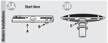
With flat side of crossbar towards ceiling, mount crossbar (A) by inserting 1/2" mounting screws (D) through holes. Screw reducer (C) into center tap. Screw 1/8 IP nipple into center of reducer Thread 1/8 IP lock nut onto nipple until it rests against reducer.
