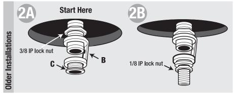
3/8 IP nipple at outlet box: Screw 3/8 IP lock nut onto existing nipple. Thread larger side of hickey (B) onto existing nipple, resting against lock nut. Screw reducer (C) into other end of hickey. Screw 1/8 IP nipple into reducer. Thread 1/8 IP lock nut onto nipple until it rests against reducer.
