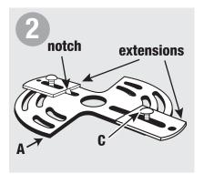
Line up notch on extension with notch on bar. Insert 3/4" screw (C) into slot on each extension and hand tighten into holes on crossbar (A). Adjust length of extensions as needed.
