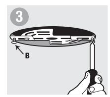
Insert 1/2" screws (B) into each hole on extension and align with holes in electrical box. Tighten all screws.
