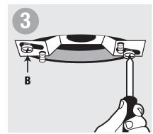
With raised side of crossbar towards ceiling, mount crossbar by inserting 1/2" mounting screws (B) through slotted holes. Tighten until crossbar is flush with ceiling.
