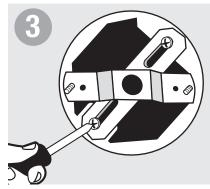
With raised side of crossbar towards opening, mount crossbar by inserting 1/2" mounting screws (not included) through slotted holes. Tighten until crossbar is flush.
