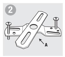
On raised side of offset crossbar (A) thread mounting screws (not included) down through each hole that lines up with fixture.
