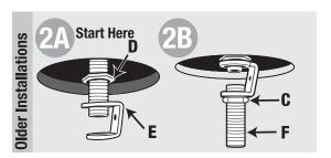
3/8 IP nipple at outlet box - Screw 3/8 IP lock nut (D) onto existing nipple. Thread larger side of hickey (E) onto existing nipple, resting against locknut. Screw 1/4 IP nipple (F) into other end of hickey. Thread 1/4 IP lock nut (C) onto nipple until it rests against hickey.
