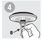
Check fit, cover outlet box with canopy and secure with screw collar loop (B). If needed, adjust nipple so canopy rests against ceiling, Remove.
