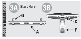
With raised side of crossbar towards ceiling, mount crossbar (A) by inserting 1/2" mounting screws (G) into slotted holes. Screw 1/4 IP nipple (F) into crossbar. Thread 1/4 IP lock nut (C) onto nipple until it rests against crossbar.
