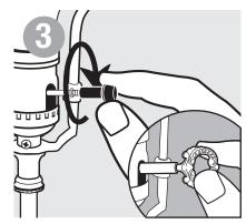
If extender was used, thread socket key or knob clockwise onto extender. Otherwise, thread socket key or knob clockwise onto socket.
