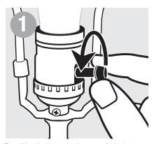
Turn old socket key or knob counterclockwise to remove from socket.
