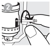
If extender is required, thread extender clockwise onto socket.
