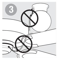
After installation make sure braided cord does not rest against lamp or interfere with fan.
