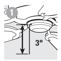
To attach use 3" of existing chain from fixture.
